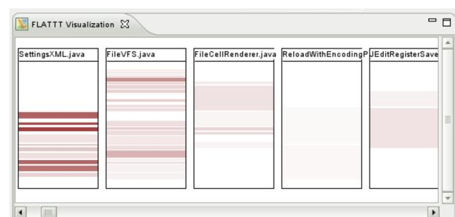
FLAT<sup>3</sup> can visualize the dispersion of a feature or search results throughout the classes of a system. The color of the highlighted rows indicates the degree of similarity of the code to the feature.
