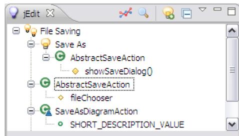
FLAT<sup>3</sup> allows the user to create and name features and then link source code to those features. These taggings or annotations are displayed in a special view. Features can be hierarchical and have sub-features. Above, *Save As* is a child of the *File Saving* feature.
