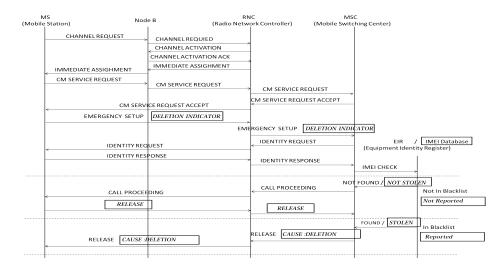
Figure 2: Emergency Call Establishment Procedure in UMTS Network
