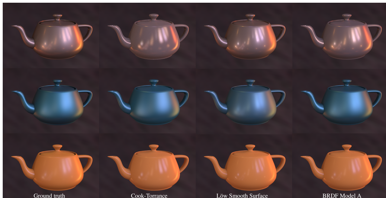
Figure 1: A comparison between Cook-Torrance [1982], Löw et al.’s smooth surface model [2012], and a new analytic BRDF model found by genBRDF, all fit with Löw et al.’s E_2 metric to three materials from the MERL-MIT BRDF database [Matusik et al. 2013].
