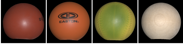
Figure 7: Homogeneous spherical objects of varying specular roughness illuminated by a frontal point light source. Left to right: red gell stress ball, orange rubber ball, green-yellow toy baseball, wooden ball.
