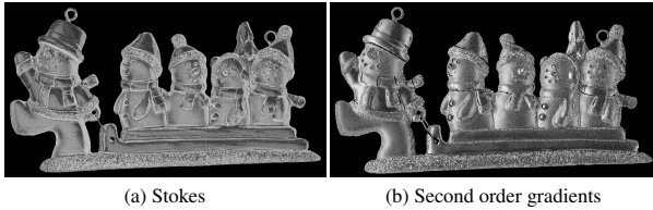
Figure 8: Comparison of estimated per pixel specular roughness with the technique of Ghosh et al. [2009]. (a) Specular roughness estimated from the Stokes measurements of constant full-on illumination. (b) Specular roughness from polarization difference imaging of second order spherical gradients.
