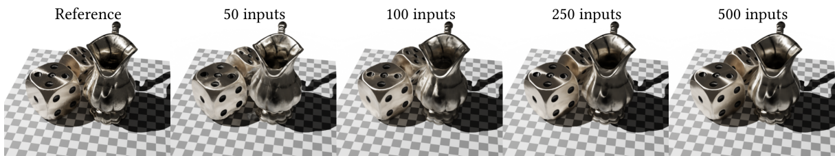
Figure 11: Impact of the number of captured training images. Increasing the number of training images improves the quality. The quality degrades significantly when the number of images is less than 250.
