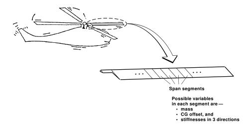
Figure 2: Rotor blade design variables
