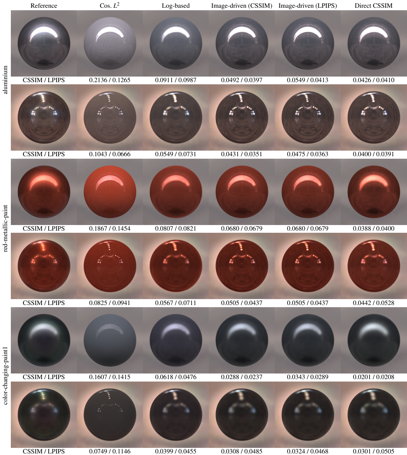
Figure 3: Image-driven BRDF fitting on three selected materials with the Cook-Torrance microfacet BRDF model compared to the classic cosine weighted L^2 BRDF fitting metric and Löw et al.'s log-based fitting metric. The CSSIM and LPIPS error is shown below each BRDF fit visualization. Note that the “Direct CSSIM” results are optimized to produce an as low as possible CSSIM error under the lighting shown. Hence it represents a lower bound on the CSSIM error for each material under the shown lighting.
