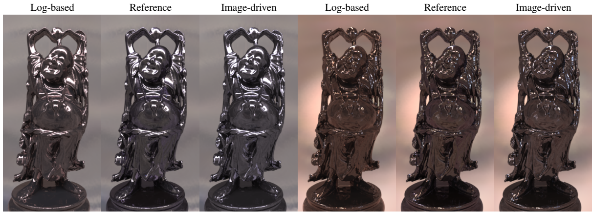
Figure 10: Comparison of log-based and image-driven BRDF fits for tungsten-carbide with the GGX microfacet BRDF model visualized on the Buddha model under the Uffizi Gallery and St. Peter's Cathedral light probes.
