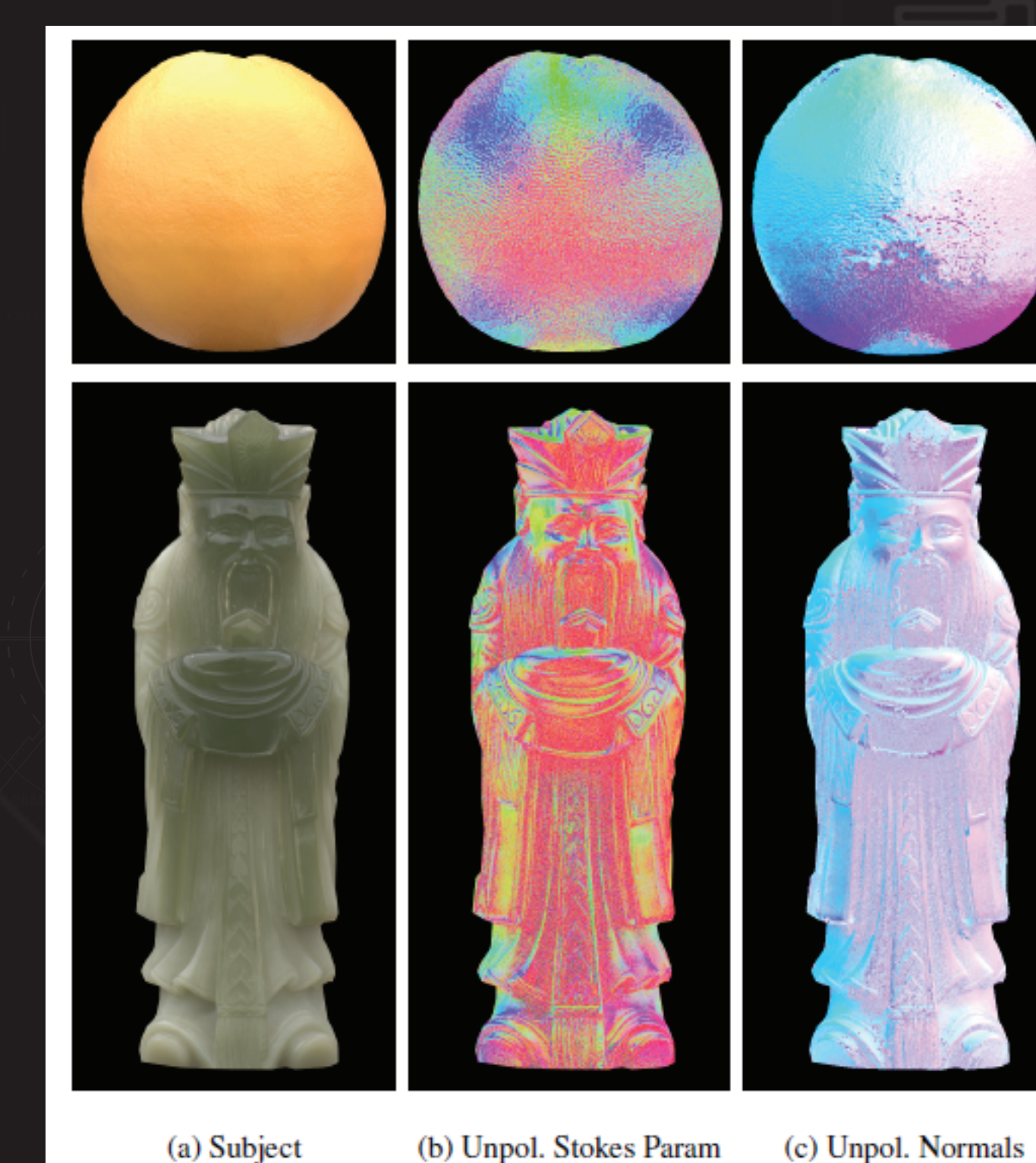
Fig. 3. Estimated surface normals from Stokes parameters of diffuse outdoor illumination. Toprow: Plastic orange. Bottom-row: Confucius statue.
