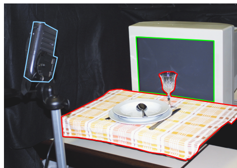
Figure 2: The scene is highlighted in red, the camera in blue and the emitter in green.
