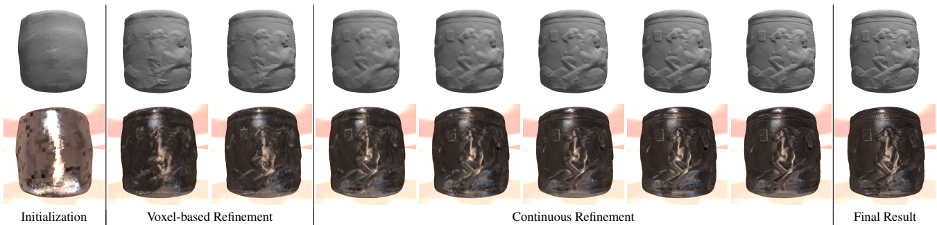
Figure 5: Shape and Reflectance Evolution. Image sequence of intermediate recovered shapes (top) and surface reflectances (bottom) for each iteration starting from the initial visual hull, followed by the voxel-based refinement results, and subsequently, the results from continuous refinement.
