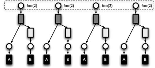
(c) Schedule of computation for blocked code after first two levels have been executed in breadth-first manner. Leaf nodes with the same label are executed as part of the same block.
