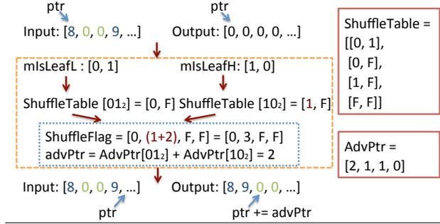
Figure 8: An illustration simulating four-way SIMD stream compaction using two-way SIMD shuffle tables.
