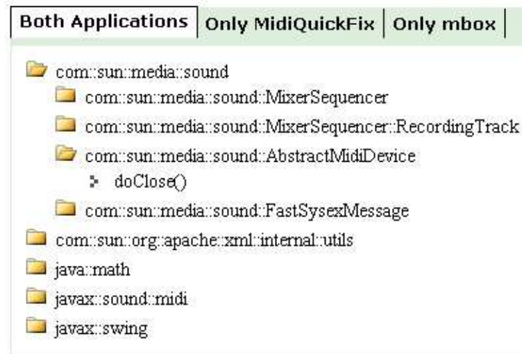
Figure 3.3: Part of the CLAN interface, showing the API calls common to two applications. CLAN shows these calls in order to help programmers concentrate on highly-relevant details when comparing applications.
