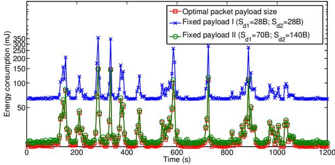
Figure 3: Energy Consumption Comparison
