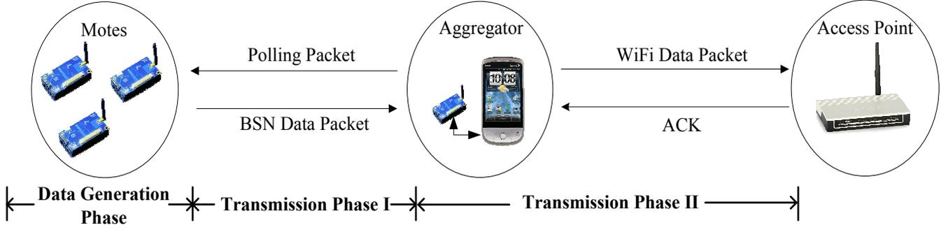
Figure 1: The Two-hop Communication System
