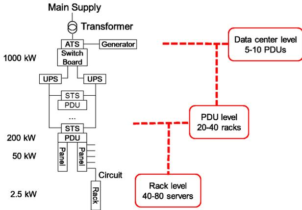
Fig. 1. A typical data center power distribution from [12]
