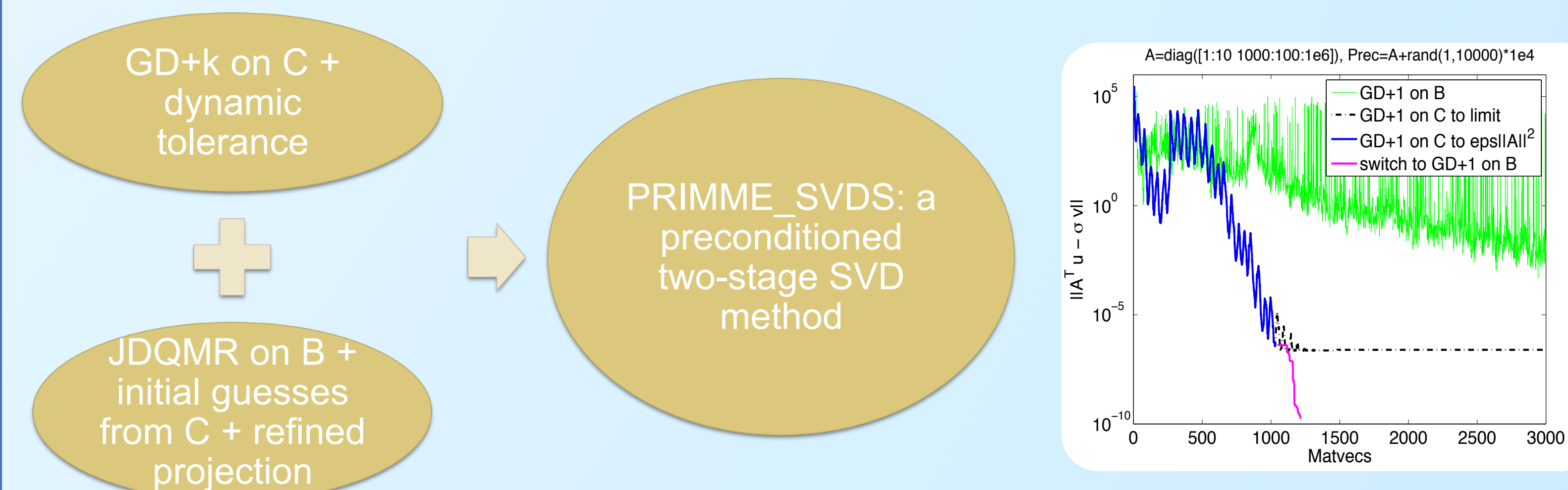
Fig. 2: Hybrid, two-stage SVD method and an example
