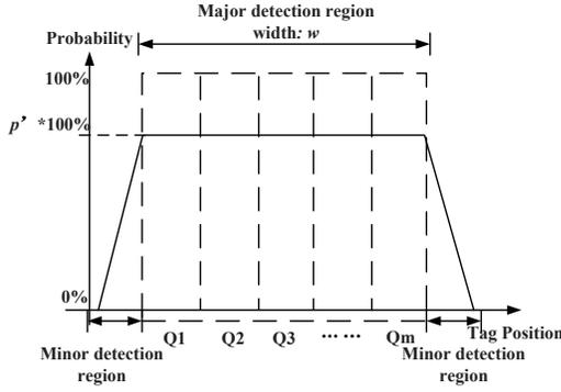
Figure 3: The model of effective scanning window
