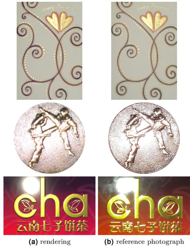
**Figure 11:** Comparison of renderings with estimated reflectance parameters with reference photographs under point source illumination from near normal incidence. (Top) Rough specular sample acquired using the flash-based approach. (Centre) Specular sample acquired with LCD-based reflectometry. (Bottom) A larger sample reconstructed using appearance transfer.
