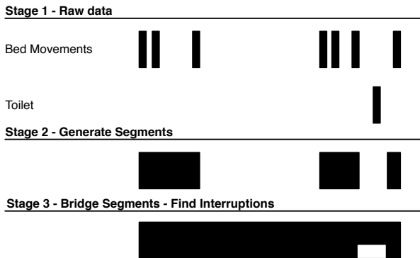
Figure 4: The discrete bed movements are processed by a multi-stage filter to discover the duration of sleeping and the number of interruptions. When other sensors fire (such as a toilet), an interruption has been created inside the sleeping segment.
