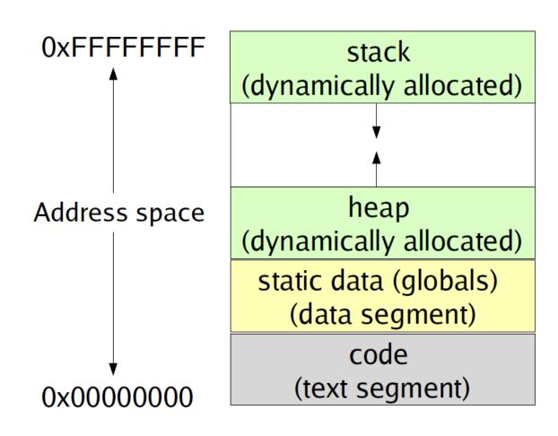
Address space is just array of 8-bit bytes
