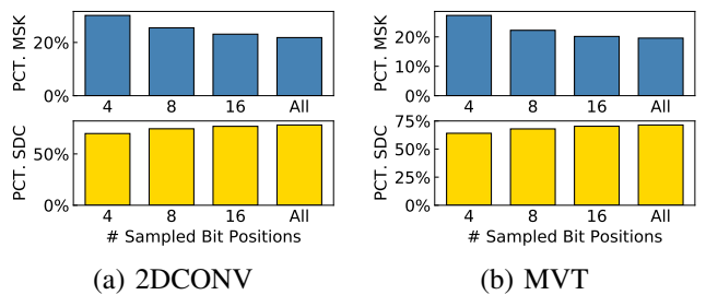
Fig. 8: Impact of bit-wise pruning on distribution of fault injection outcomes for (a) 2DCONV and (b) MVT (all registers). Percentage of outputs stabilizes at 16 bits.
