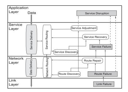
Fig. 3. A Service Composition and Recovery Framework in a Mobile Ad Hoc Network
