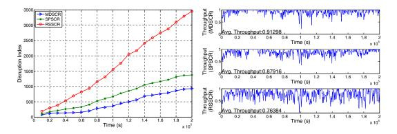
Fig. 9. Disruption Index for MDSCR, SP- Fig. 10. Throughput for MDSCR, SPSCR, SCR, and RSSCR When Service Path and RSSCR When Service Path Length is Length is 4 Using CBR Traffic 4 Using CBR Traffic
