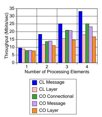
Figure 5: Process Architecture Throughput
