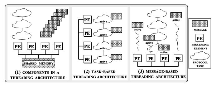
Figure 1: Basic Process Architecture Components and Interrelationships
