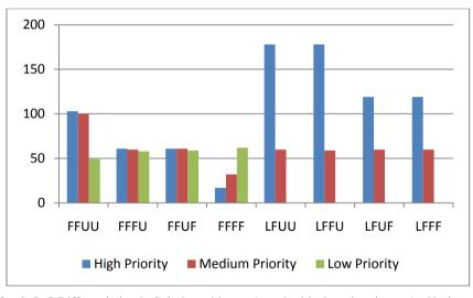
Fig. 6. QoS Differentiation in Solution with  $t_m = 1s$  and critical section time = 1s. Horizontal access shows the Priority-Request-Reply-Release models that were being evaluated. Vertical axis indicates number of mutexes entered.
