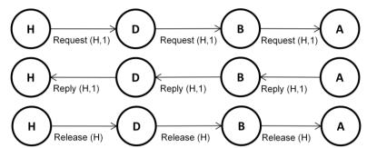
Fig. 4. Messaging Required for a Critical Section Entry from Participant H to a Logical Root Participant A (Diagram Assumes a Forward-Forward Configuration).
