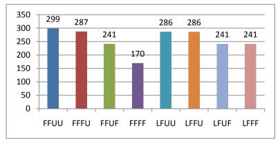
Fig. 9. Total critical section entries in solution with  $t_m = .5s$  and critical section time = 1s during a 360s test. Horizontal access shows the Priority-Request-Reply-Release models that were being evaluated. Vertical axis indicates number of mutexes entered.
