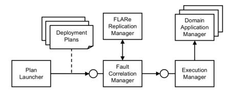
Figure 6: FaultCorrelationManager Integration into the D&C Infrastructure
