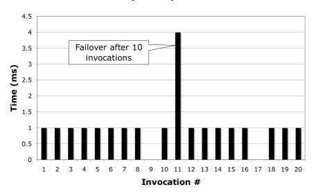
Figure 11: Single Fail over Latency Measurement
