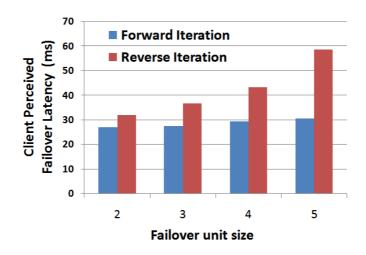
Figure 15: Client Perceived Fail over Latency When the Tail Component Fails
