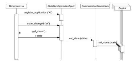
Figure 8: State transmission sequence based on a common interface
