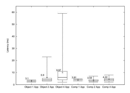
Figure 12: Results for Failover Latency Measurements
