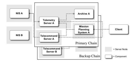
Figure 1: Component-Based Mission Control System
