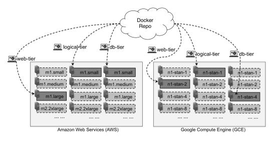
Figure 3: ROAR's Deployment Manager Pulls Applications from Docker and Deploys Them to Servers in Different Cloud Platforms
