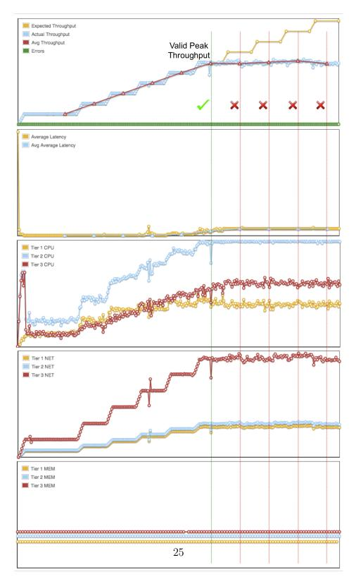
Figure 4: A Sample Test State Model with Aligned Data on Throughput, Average Latency, CPU, Memory, and Network
