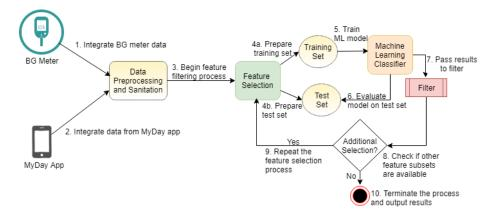
Figure 1: Iterative Process of Our Learned Filtering Architecture (LFA).
