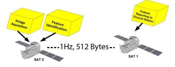
(b) A Software Deployment Topology Using Two Nodes and Less Bandwidth
