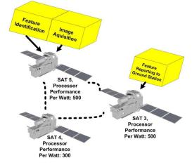
(b) A Software Deployment Topology for the Fractionated Spacecraft with Superior Performance per Watt
