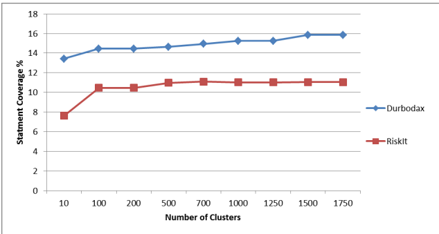
Fig. 8: Dependency of the statement coverage on the number of clusters for subject applications.
