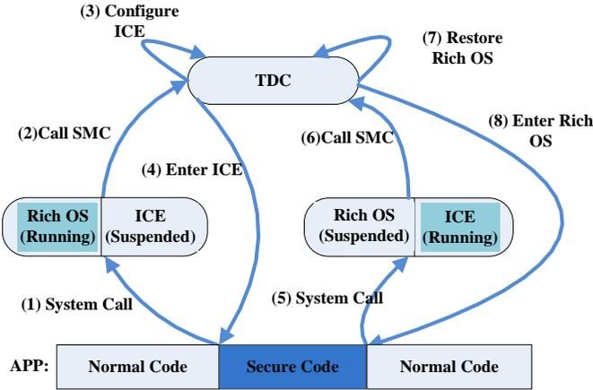
Fig. 7: Switching between Rich OS and ICE
