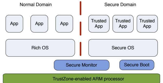
Fig. 1: Traditional TrustZone Architecture
