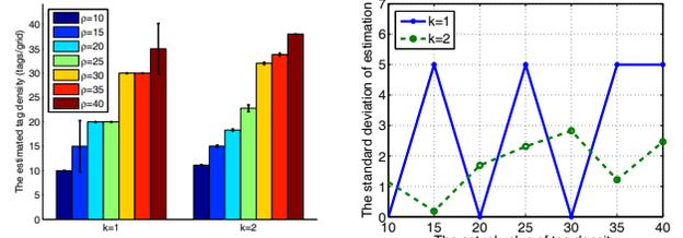
(a) The average value and (b) The estimation error of standard deviation for estimated tag density
