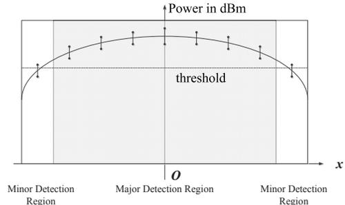
**Figure 2: The average value and variance of the incident power in the one-dimensional space: a schematic diagram**
