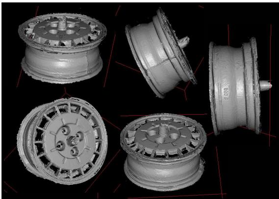
Figure 13: A reconstruction of a specular metal wheel.
