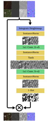
Figure 2: Network architecture used for the mixture augmentation.
