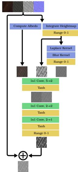
Figure 1: Network architecture used for the roughness augmentation.
