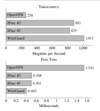
For both metrics, WireGuard outperformed OpenVPN and both modes of IPsec. The CPU was at 100% utilization during the throughput tests of OpenVPN and IPsec, but was not completely utilized for the test of WireGuard, suggesting that WireGuard was able to completely saturate the gigabit Ethernet link.
