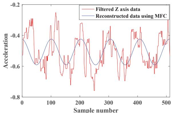
Fig. 6. Noisy acceleration data and reconstructed data using MFC
