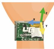
Fig. 4. UG Device Deployment on Wrist
